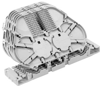
FIST™ Splice Sub-assembly kit with 8 slim element trays, each for holding up to 12 primary coated fibers, with Heat Shrink type splice holder
